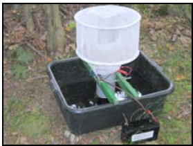
A gravid trap is used in our West Nile Virus Surveillance Program.
